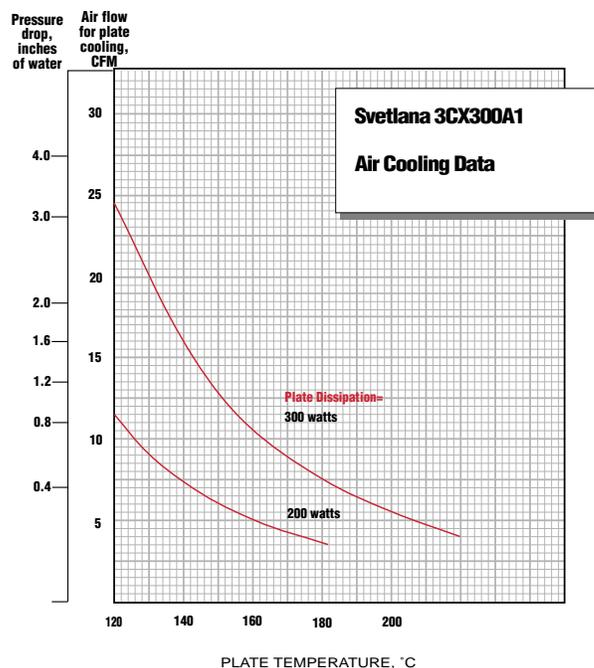
The flow rate for base cooling must be determined for satisfactory cooling to obtain base temperature not more than 220°C.
